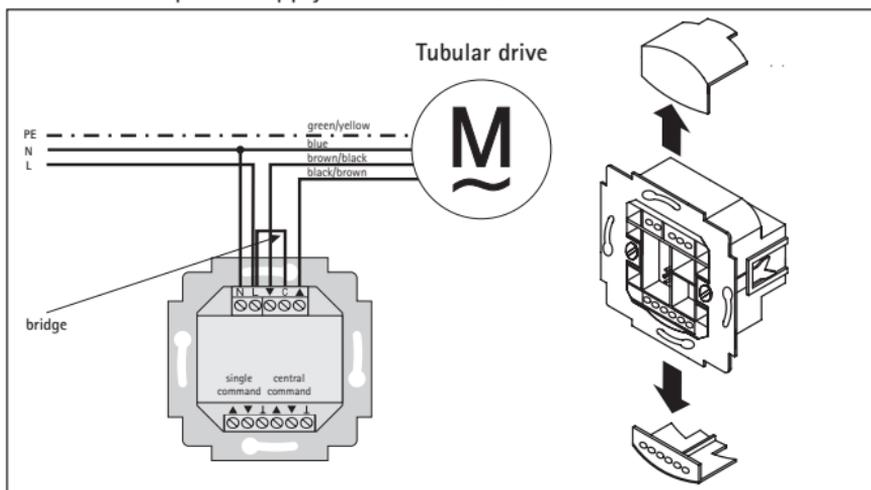
2. Put the protective caps back on the power supply unit.
